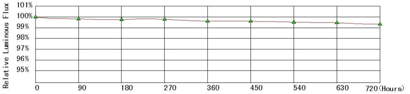
Through 720h accelerated aging test, high and low temperature prediction in the rated under the working condition after 3500h, will provide an average 70% optic maintenance ratio(L70).
